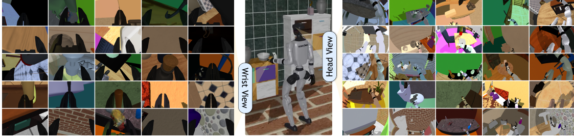
Figure 2: Simulated observations. Example frames of the head-fisheye and wrist streams the policy receives, across scenes randomized in texture, lighting, and camera intrinsics and extrinsics.
