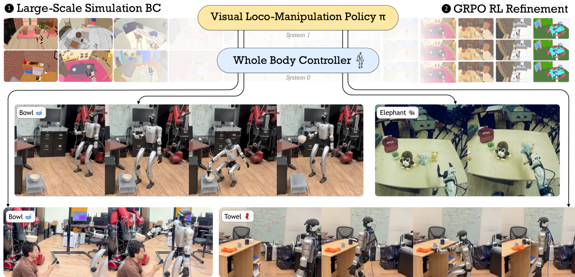
Figure 1: FETCHMAN learns visual humanoid loco-manipulation entirely in simulation and deploys it zero-shot to a real Unitree G1. The resulting policy walks up to and grasps objects across diverse, unseen real-world scenes, with no real-world data or per-scene tuning.
